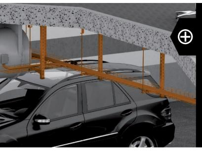
If a fire breaks out in an underground car park, it can quickly lead to the development of an enormous level of smoke. For safe evacuation, the operation of smoke extraction systems must therefore be guaranteed. Through the extraction of the developing heat, the entire building structure is simultaneously protected. And, of course, with good smoke extraction, fire brigades can better localise the centre of the fire.
