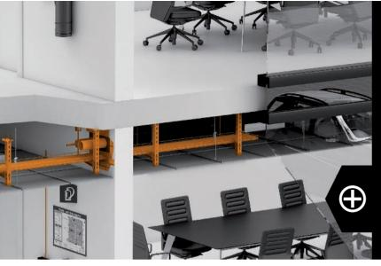
With installations above suspended fire protection ceilings, particular care is required: If there is a fire, the ceiling must not be stressed or damaged by falling or deforming parts. Cable support systems used here must be designed to be safe in the event of fire and offer a large selection, in order to adapt themselves optimally to the cable volume to be routed and to the available installation space.
